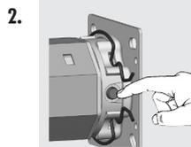
Activate connect / disconnect mode on the DuoFern tubular motor by briefly pressing the set button (7).
