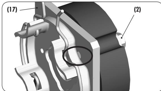
2. Subsequently slide the bearing block (3) back onto the cross member (18) of the awning until the drive bearing (4) fully engages on the drive head (6) (see Fig. ⑦).
