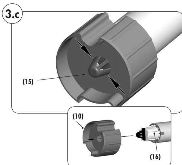
1. Press the side parts of the retaining clip (15) together and pull the catch (10) off of the drive adapter (16).
