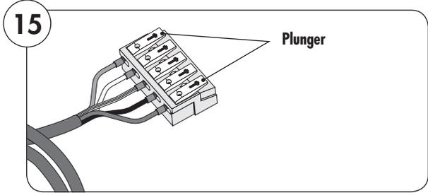
Open the terminal contacts by pressing the plungers and connect all of the wires of the motor cable (13) as follows:
