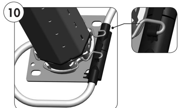
The retaining spring (5) should be rotated 90° to be plugged in and re-engaged.
