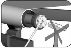
**Never knock the motor (9) with force into the awning shaft (11).**
