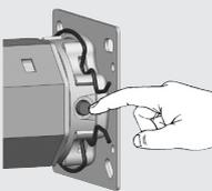
Press and hold the set button (7) on the motor until the lower end point is reached.
