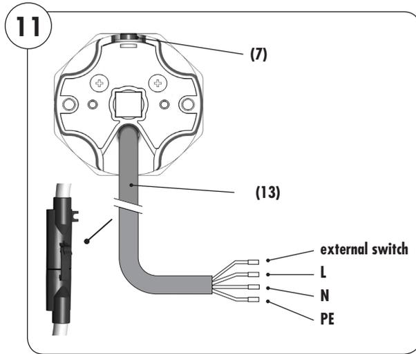
1. Connect the motor cable (13) to the connecting cable supplied by means of a connector and make the connection according to the following wiring configuration.
