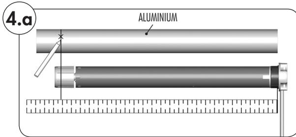
1. Measure the distance between the adapter (8) and the rear third of the catch (10) and mark this distance on the precision tube.
