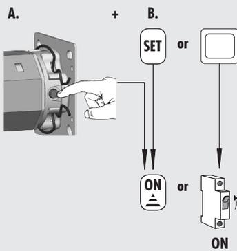
First press and hold the set button (7) on the tubular motor (9) and subsequently press and hold the SET button on the cord circuit setting device (20) (possibly a second person carries this out).
