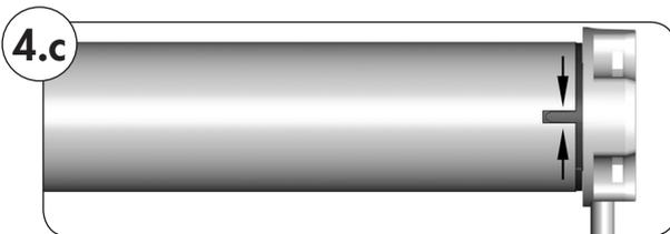
3. Slide the tubular motor (9) into the precision tube.
