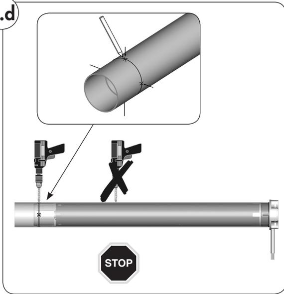
4. Mark the four fastening holes and subsequently drill them through the precision tube in the catch (10).
