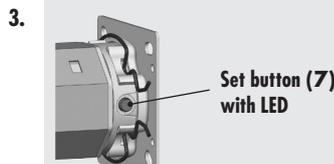
The DuoFern tubular motor is briefly running up and down and the motor set button (7) lights up orange by way of acknowledgement.
