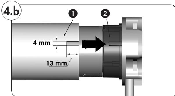
2. Saw a groove in the end of the precision tube ① in order that the cam ② of the adapter (8) can be completely pressed into the tube.
