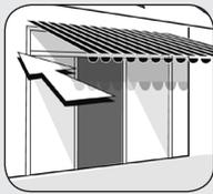
The awning will first retract to the upper stop until the tubular motor switches off automatically.
