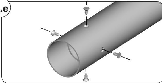
5. Screw or rivet the precision tube to the catch (10).
