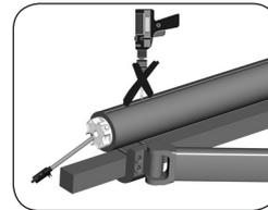
**Never drill or insert screws in the area of the drive. Doing so may damage the tubular motor.**
