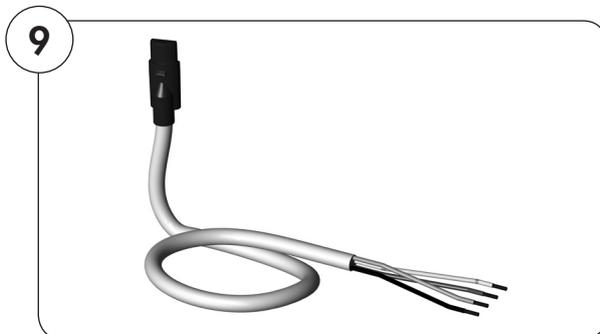
The plug connection can be fixed to the drive bearing if required to secure the cable.
