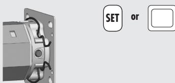
Release the set button (7) on the tubular motor (9) and the SET button (or the external switch, if connected).
